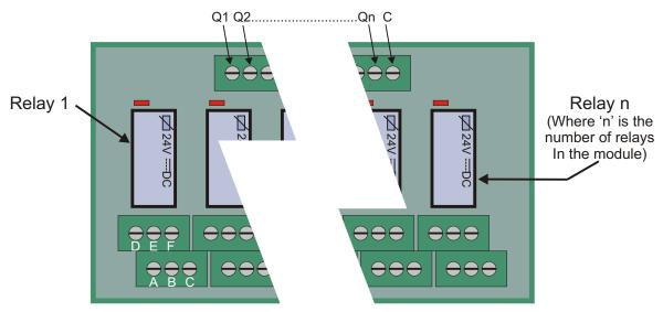
Connections to the relay contacts are made by the terminals A,B,C,D,E,F. Each relay is connected in the same way:
