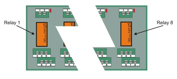
Terminals 3,4,5,6,7 & 8 on each relay are the contact connections.
