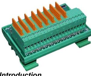
DIN - Rail mounting power distribution module Provides 8 individually fused supply lines LED indication of fuse integrity Avoids looping of power cables between devices
