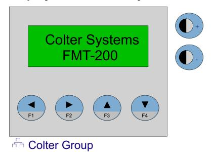
The FMT-200 range of controllers incorporates a two line by sixteen character LCD display. The display is treated by the FMT as serial port 8.
