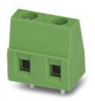
PCB terminal block, Nominal current: 17.5 A, Nom. voltage: 630 V, Pitch: 7.5 mm, Number of positions: 2, Connection method: Screw connection with tension sleeve, Mounting: Wave soldering, Conductor/PCB connection direction: 0 °, Color: green, The article can be aligned to create different nos. of positions!
