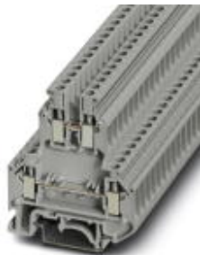
Double-level terminal block, Connection type: Screw connection, Cross section: 0.2 mm 2 - 4 mm 2 , AWG: 24 - 12, Width: 6.2 mm, Color: gray, Mounting type: NS 35/7,5, NS 35/15, NS 32
